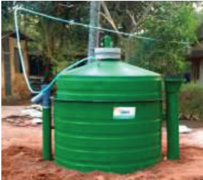
PORTABLE BIOGAS PLANT
