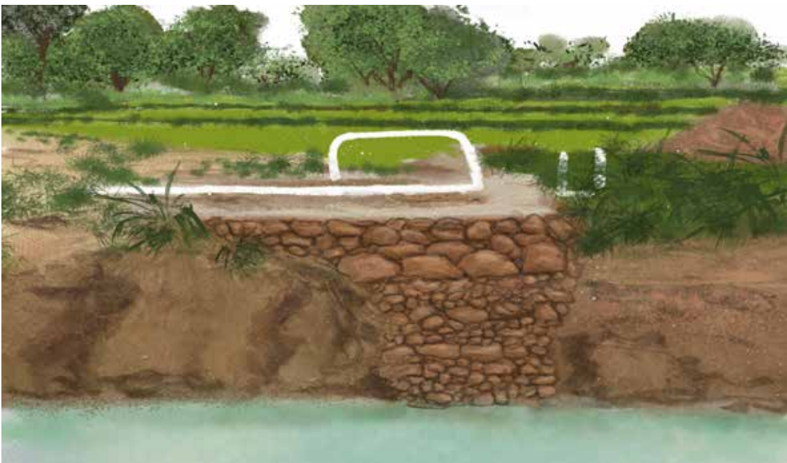
Figure 8.25: Borewell recharge using pond
