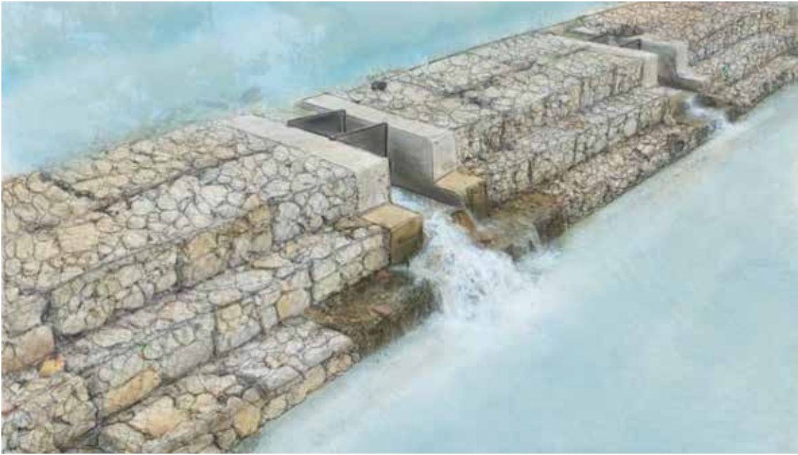
Figure 8.13: A Gabion structure across a stream with weir plates to regulate flow and arrest soil erosion
