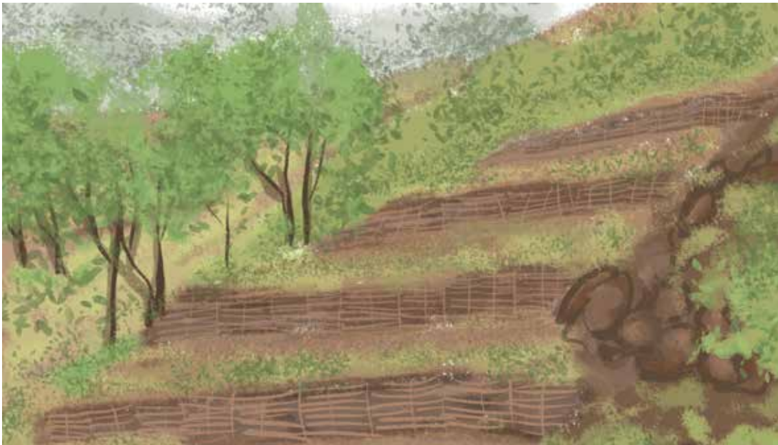
Figure 5.8: Bamboo fencing on a slope
