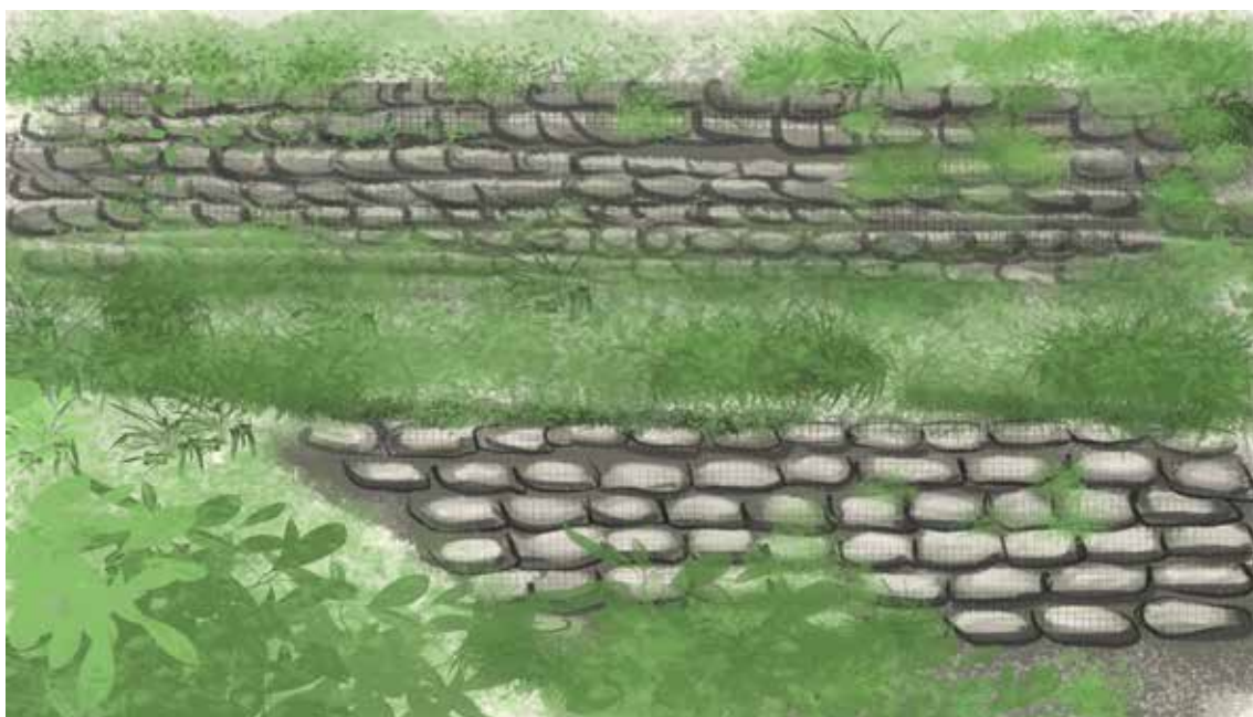
Figure 5.12: Vegetated soft gabion wall
