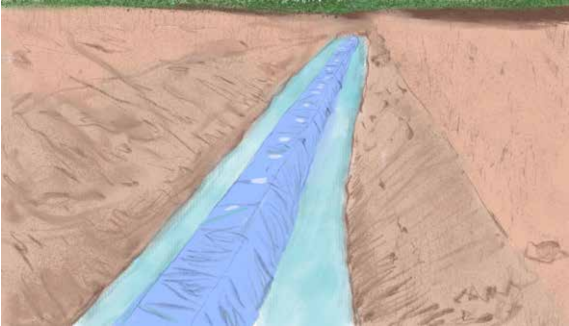
Figure 8.19: A subsurface dyke constructed across a dry alluvial river bed to recharge and hold groundwater upstream
