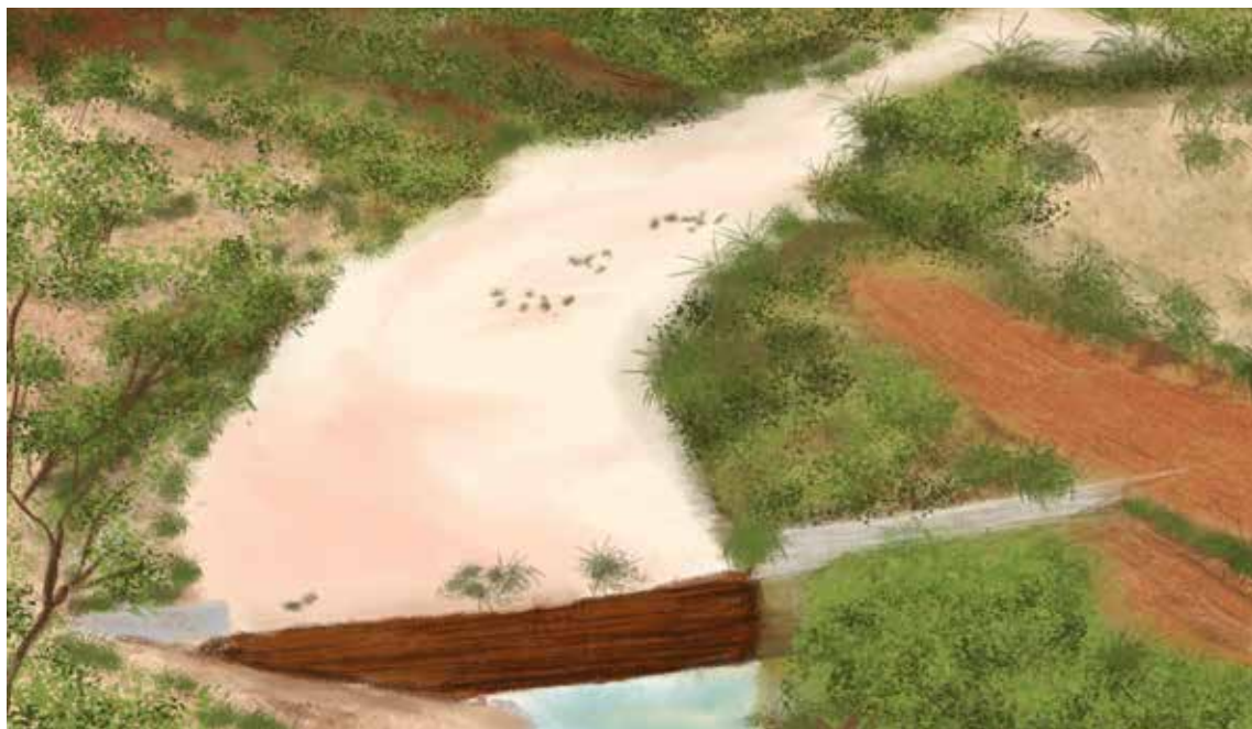
Figure 8.21: A sand dam constructed across a dry river bed, wherein groundwater is held in the sediments upstream
